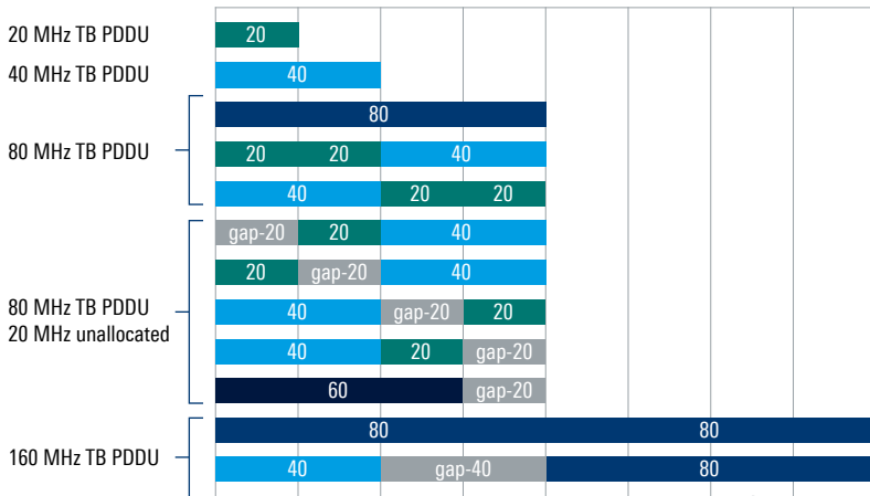
Figure 5: DBW modes for the 20 MHz TB PPDU, 40 MHz TB PPDU, 80 MHz TB PPDU and 160 MHz TB PPDU
