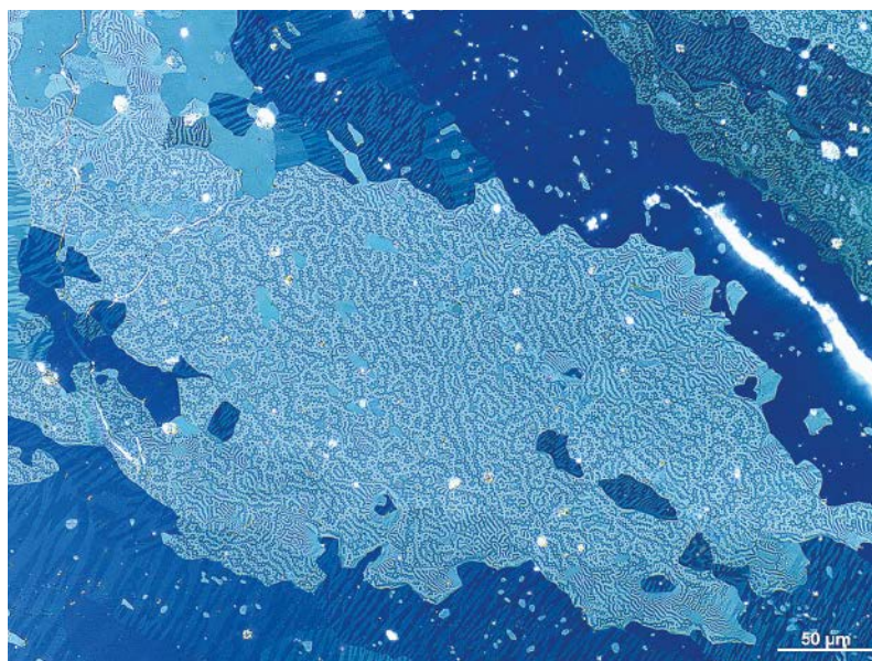
Figure 2: Kerr microscopy micrograph of a permanent magnet used in new electric vehicle motors. Colors indicate magnetic domain orientations.
