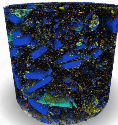
3D rendering of powdered black mass (recycled battery) materials. Microscopic data acquired by ZEISS VersaXRM, segmentation and rendering by Dragonfly. Blue represents the NMC cathode materials, turquoise the Cu foil, red the LFP cathode, green the Al foil, yellow the polymer separator, and black the graphite anode.
