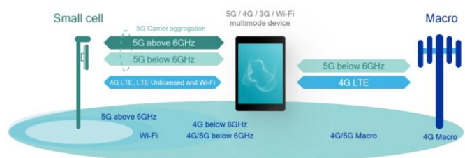
Fig. 3. The 5G multi-connectivity concept. Source: www.qualcomm.com
