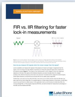
When characterizing a device, you often look for a small response to some sort of stimulus. Frequently, this is being done in the presence of a DC offset as well as a lot of noise — which often can be larger than the signal itself. The typical way to obtain the sought-after level of response is to use a lock-in amplifier.
