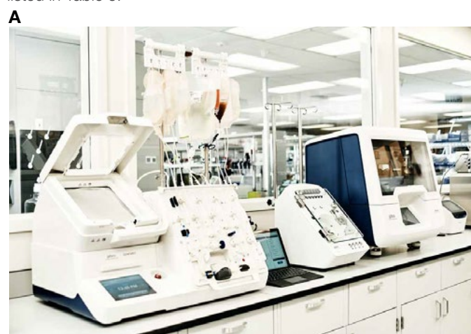
Figure 1. T cell isolation process summary. T cells were isolated using the CTS DynaCollect system and then cultured in CTS OpTmizer Pro SFM with 100 U/mL IL-2 for 3 days. Following bead removal on day 3, T cells were washed and then transferred from the CTS Rotea system to the CTS Xenon system via a closed integration. (A) The CTS DynaCollect system, the CTS Rotea system, and the CTS Xenon system (from left to right) are shown. (B) Schematic representation of the physical integration via a welded PVC line between the CTS Rotea system and CTS Xenon system used for T cell electroporation on day 3.
