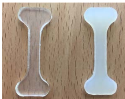
Fig. 3: TPU reference (left) and TPU prepared with 6.2% glucan (right).
