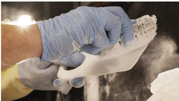
These 3D-printed insoles from Wiiv Wearables are one example of customized products designed, developed, and created using additive manufacturing.
