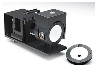
Figure 8: Integrating sphere from a diffuse reflectance accessory, with detector at bottom
