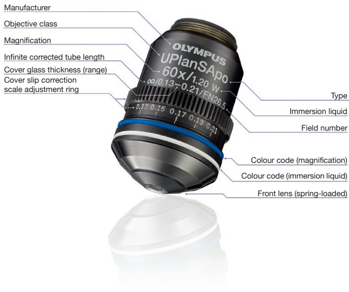
Figure 6. Lens barrel showing the inscriptions detailing the lens properties. Copyright Olympus.
