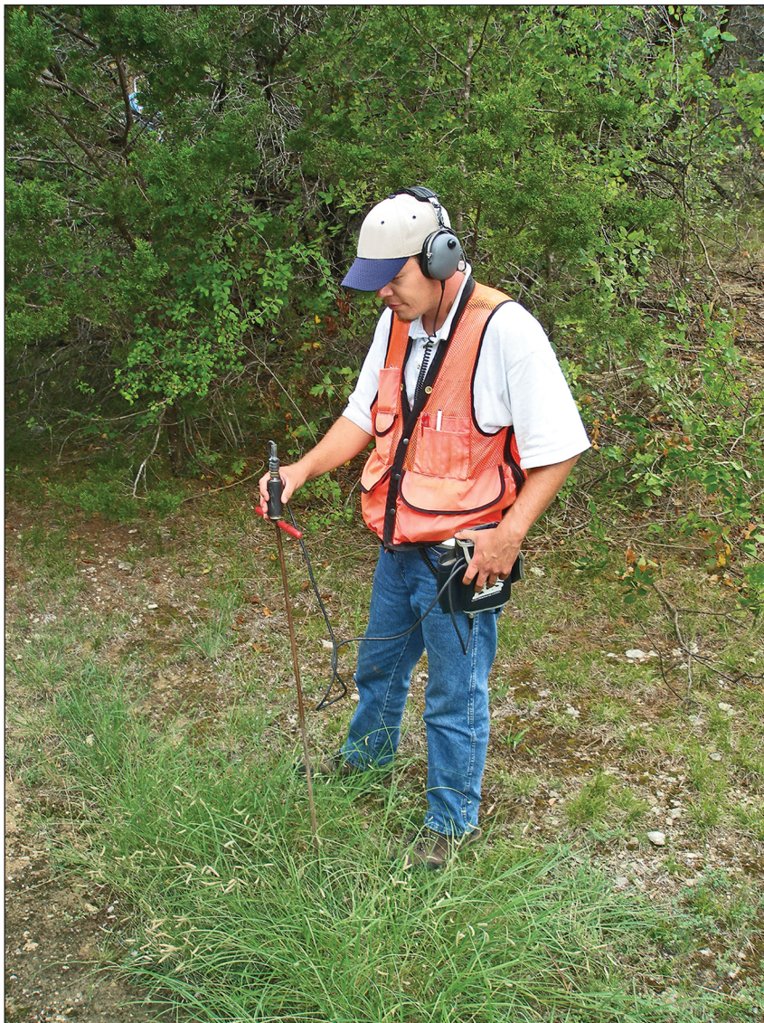
Acoustic devices allow users to detect the presence of leak noise and accurately pinpoint leak locations quickly. Photograph: M.E. Simpson
