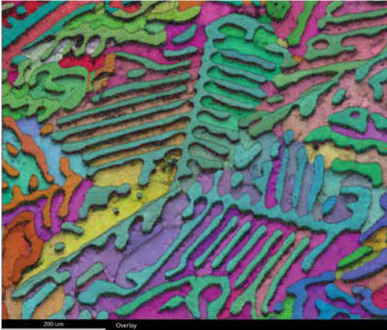
Fig 3. Orientation map of a aluminum-germanium dual phase material
