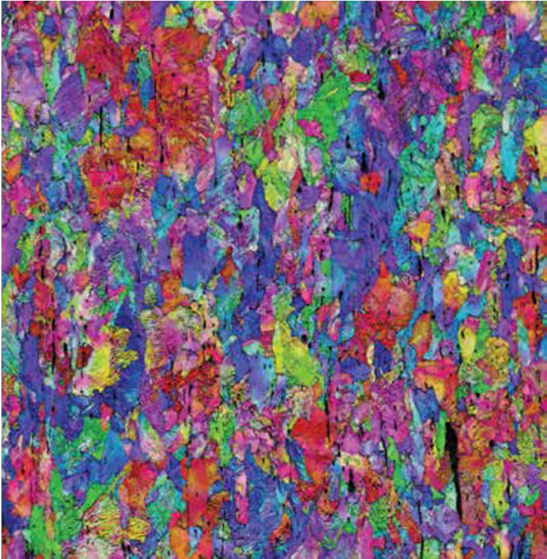
Fig 9. Orientation map of a deformed pearlitic steel alloy
