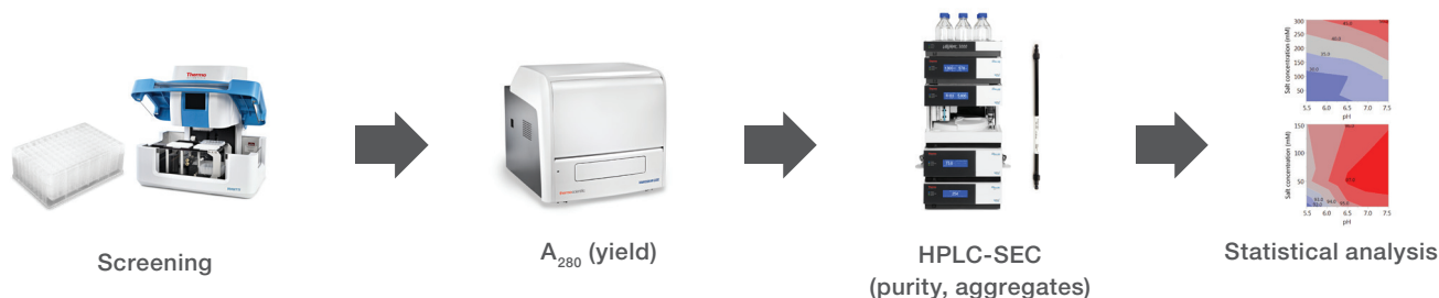
Figure 3. The general workflow for aggregate removal consists of filter-plate screening followed by A_{280} concentration determination and purity analysis by HPLC-SEC; statistical analysis is used to generate trends and to select process conditions.
