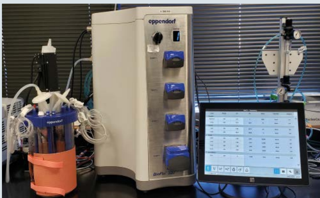
Fig. 1: BioBLU 3c Single-Use Bioreactor (left) and BioFlo 320 bioprocess control system (right).
