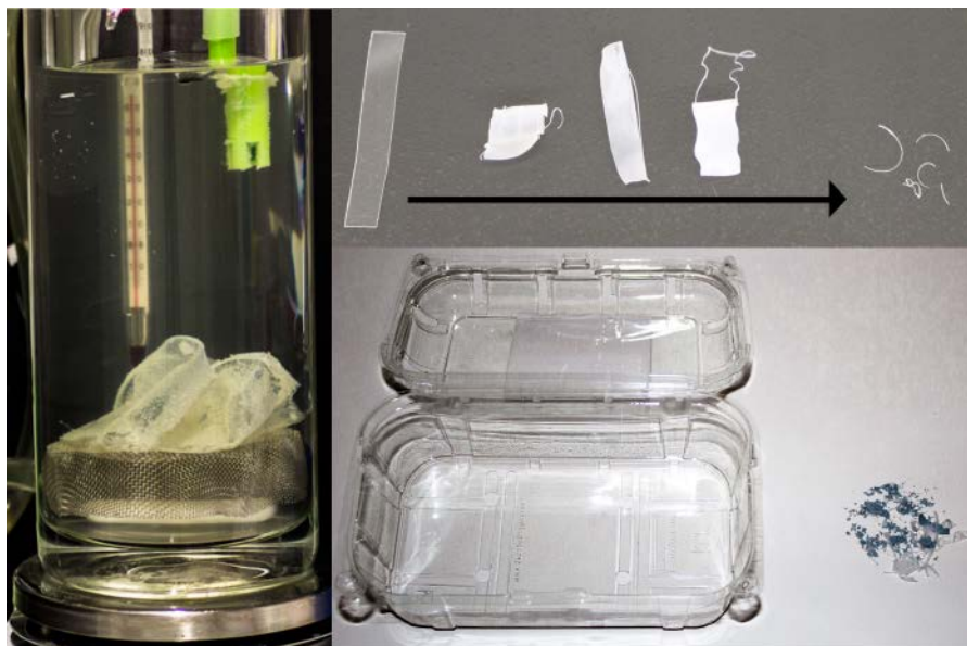
Fig. 1: Enzymatic depolymerization of PET thermoform packaging.
