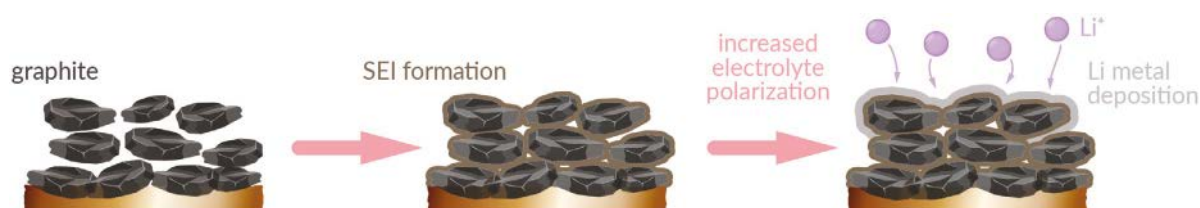
Figure 7. Illustration of SEI growth and pore-clogging during cycling inducing polarization and therefore promoting Li metal deposition.
