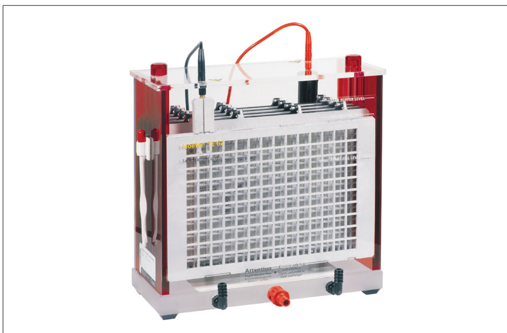
Figure 8.3.2 Large gel tank electrotransfer unit. Designed for larger 15 × 21-cm gels, these units will process four gels at a time. Note that the two outside panels hold the electrode grid. Figure courtesy of Hoefer, Inc.
