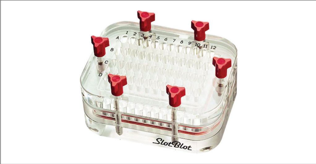
Figure 8.3.3 Slot-blot unit. Through use of a vacuum manifold or by simple hand spotting, up to 96 samples can be applied to a single NC or PVDF membrane for immunoblotting analysis. Although this approach cannot discriminate between the protein of interest and a cross-reactive antigen, it is a quick way to perform preliminary characterization and high-volume, routine quantitation of a sample. Figure courtesy of Hoefer, Inc.
