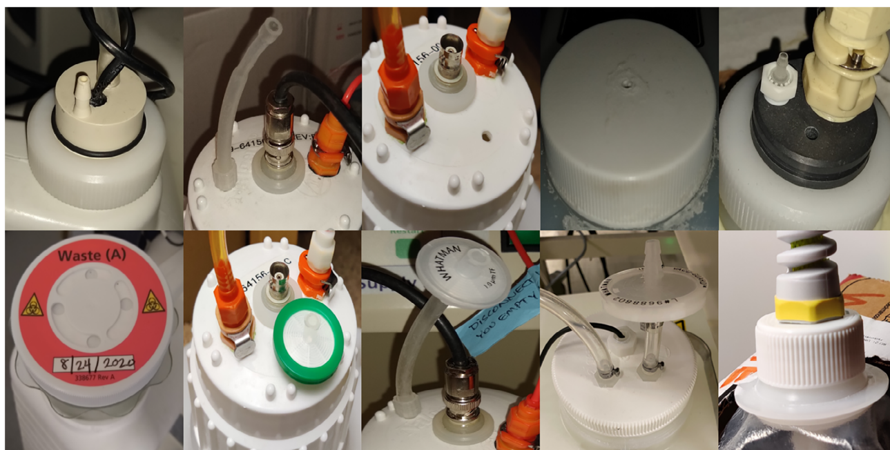
FIGURE 3 Waste tank caps. All instruments except bottom right have clear vent holes. Top row demonstrates instruments lacking air filters within vent holes. Bottom row demonstrates instruments with air filters placed within vent holes [Color figure can be viewed at wileyonlinelibrary.com ]
