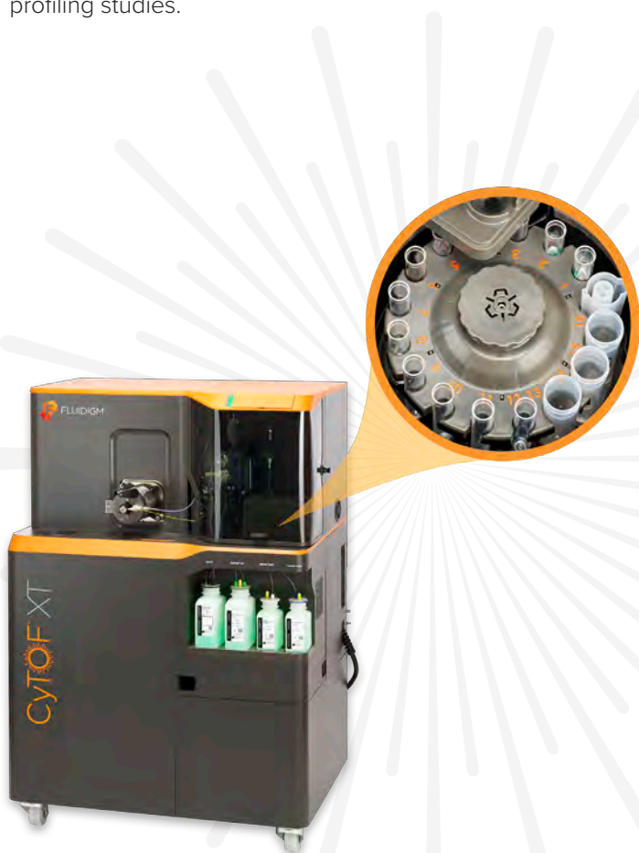
Figure 1. CyTOF XT, featuring a streamlined design and automatic sample acquisition.
