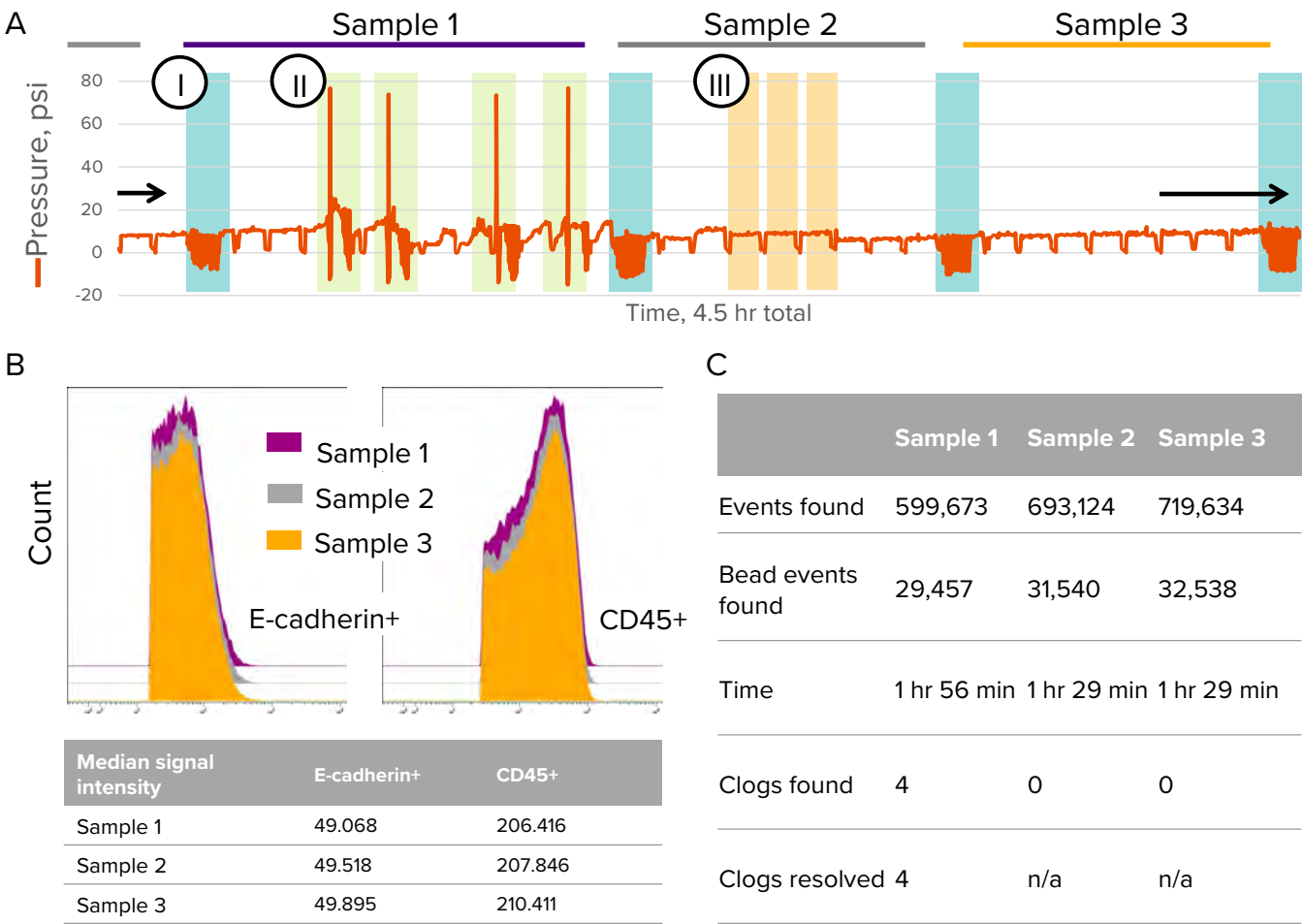
Figure 4. Automated unclogging by CyTOF XT resolves blockages with no impact on data quality. 12 samples (2.5 mL each) were acquired automatically with several occurrences of high pressure due to multiple clogs in single samples. A) Pressure monitoring of the 12 samples identified 3 consecutive samples with varying unclogging routine experiences. Section I (light blue) denotes washing steps between samples. During this time, rapid pressure swings are observed as positive to negative pressure readings, which function to remove the remaining sample in the line. Similarly, pressure during the unclogging routine (Section II, light green) fluctuates to effectively remove the clog and enable the continuation of the acquisition. A rhythmic pattern (Section III, light orange) in the pressure readings is seen in the acquisition of Sample 2 and Sample 3. This pattern is caused by the change in pressure detected between single loops of a sample that are loaded into the Autosampler module. The loop accommodates 250 \mu L of the sample volume and the entire acquisition happens in intervals, hence the rhythmic pressure pattern. B) The automatic unclogging routine did not impact signal intensity, as illustrated by the unchanged signal intensity of 2 major populations between all 3 samples. C) Summary of collected events and detected clogs.
